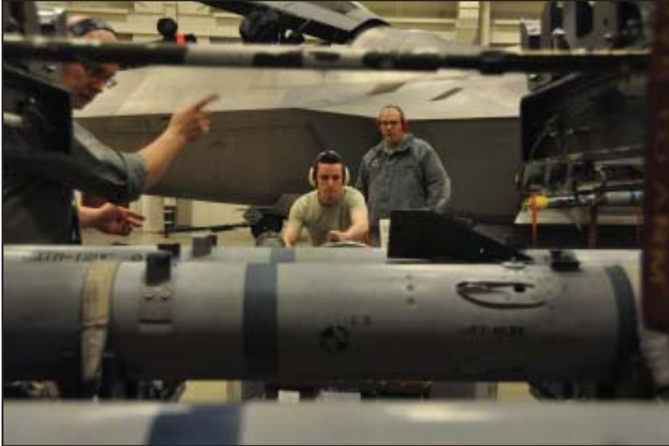
Tech. Sgt. Anthony Cords evaluates Senior Airman Joshua Baker as he picks up an AIM-120 air-to-air missile with a jammer while Tech. Sgt. Timothy Tuttle gives him directions during the 2012 JBER F-22 Weapons Load Competition. Tuttle and Baker are both Reserve weapons loaders assigned to the 477th Aircraft Maintenance Squadron. Their three man crew was recently awarded the 2012 JBER F-22 weapons load crew of the year. (U.S. Air Force/ Tech. Sgt. Dana Rosso)
